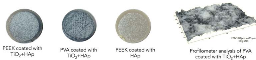
FIG. 7: Plasma-sprayed polymer samples using a plasma power of \sim 42 kW. Also shown is an optical profilometer graph of one of the samples.
