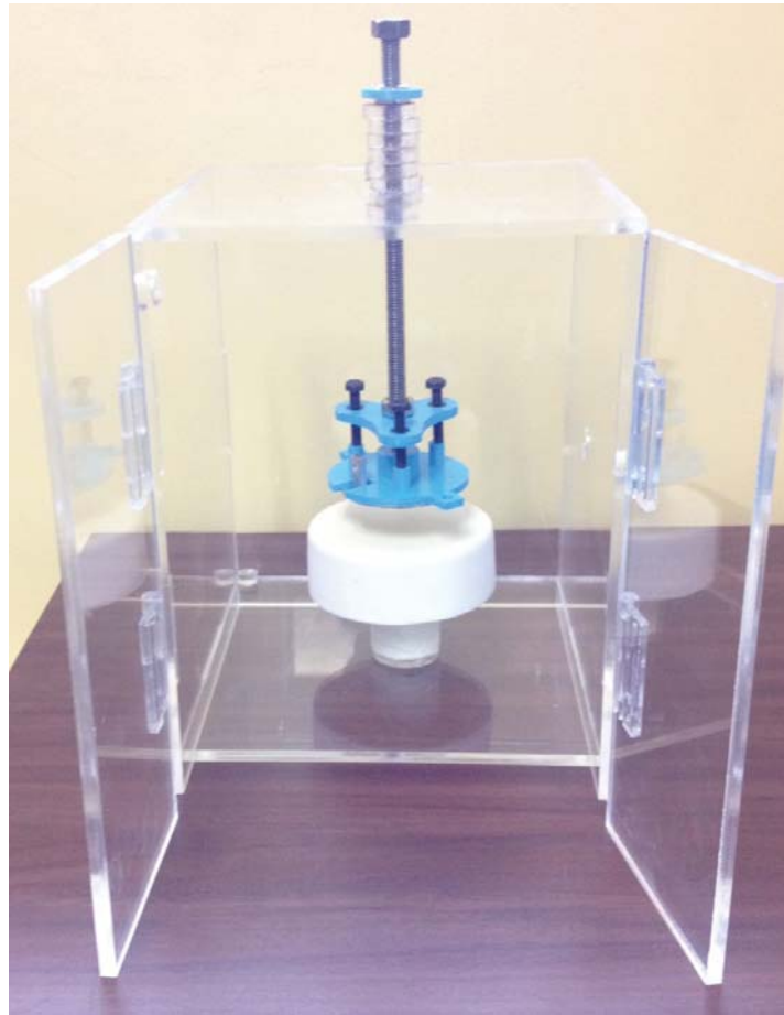
FIG. 5: DBD device developed for the studies of in vitro cultured murine fibroblasts irradiated with APNP
